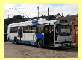
Chassis: Renault ER100 **Chassis No:** 4 ELC 2330 T Motor: Renault B34D+72 **Bodywork:** Length: Width: **Body Number: Unladen Weight: Entered Service:** 1980 Withdrawn: 2004 **Owner:** The Trolleybus Museum at Sandtoft
