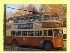
Chassis: Chassis No: Motor: Bodywork: Length: Width: Unladen Weight: Entered Service: Withdrawn: Owner: Sunbeam W4 Sunbeam W4 50393 British Thomson Houst N.C.B. H30/26R 26ft 7ft 6in
