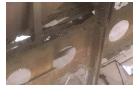
Above: The joint between the upper and lower deck structure on the near-side (this was the better side!), viewed from the outside: the rotten floor planking had disintegrated such that the whole upper deck structure had dropped by over 1½” so that the upper and lower deck pillars were touching each other. New stress panels
