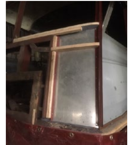
Above: The staircase rebuilt – the original inner stringer and one riser were salvaged and repaired but other parts had to be fabricated using old bits as a pattern
