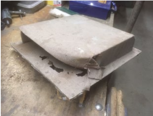
Above: One of the old roof vents, well battered and rusted
