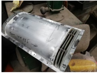
A newly-fabricated replacement roof vent (DS)
