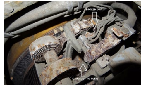
A view through the top inspection panel of the traction motor casing on South Yorkshire 2450. What remains of the commutator brush springs can be clearly seen.
