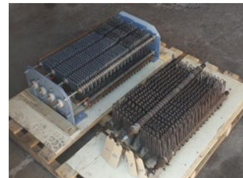
Bournemouth 99's refurbished resistance bank (left) with the innards of the old one (BC)
