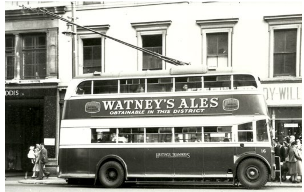
In its original livery Hastings 16 (BDY 791) is a 1940 AEC with Park Royal body. 11-20 were said to have Weymann frames, due to the outward curve on the skirt rail, but this is not proven in any documentation. (Author's Collection)
