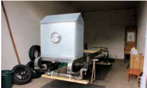
The chassis, with the front dashplate surmounted by the removable sloping cowl. "Keighley" is painted in red on the front of the chassis.
