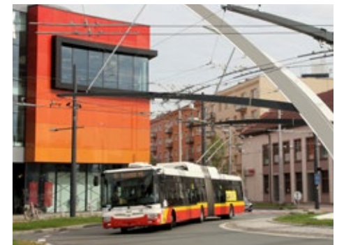
One of Hradec Králové's Škoda 31 Trs, No 69, emerges from Puškinova to negotiate a roundabout with a large artwork from which the trolleybus overhead is suspended.
