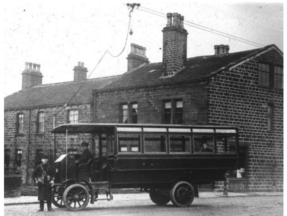
Another view at Lees (Cross Roads) in 1913, but seemingly after the line opened for service. The current collection method is well shown. The terraced houses in the background still exist. (British Trolleybus Society Library)
