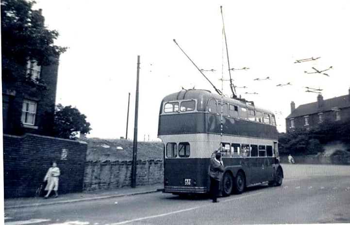
Driver Laurie Johnson re-attaches the booms of Rotherham 30 (FET339) at the junction of Park Lane and Hollings Lane, Thrybergh. It appears to have dewired at the frog which would have enabled it to go to Silverwood Colliery on route 49 - a branch off the main line Route 6 to Thryborough
