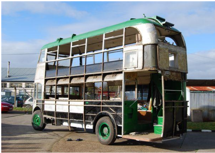
Ipswich 105 in November 2008 stripped of panels and with most of the electrical equipment missing and trolley gear removed
