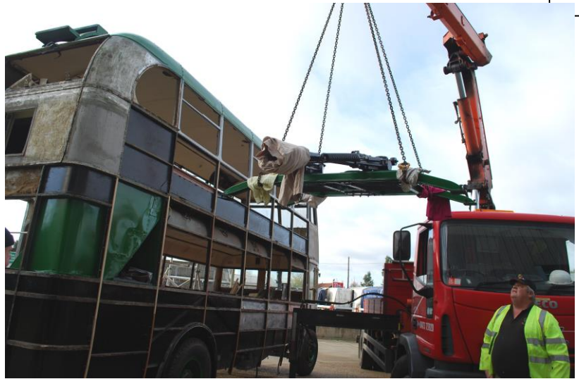
The renovated trolley gantry unit being carefully manoeuvred into place Photo: ITM collection
