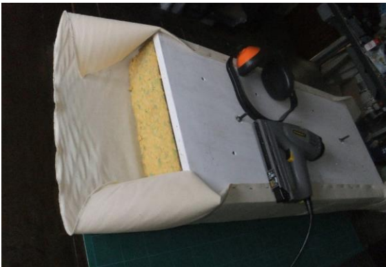
The new seat cushion for 493 takes shape as the interior foam is glued to the base and covered with calico
