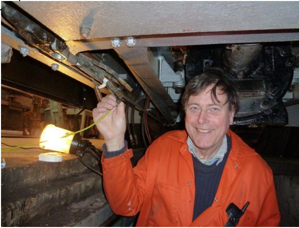
Len Smith under 375 working with Bruce Lake to determine which wire connects to which between the traction motor and the contactor box
