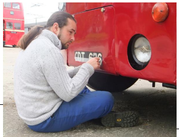
Below: Kieran Proctor un.masks the registration on the repainted front panel (4 May)
