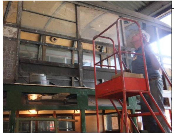
John Whipham assesses the condition of the exposed wooden framework
