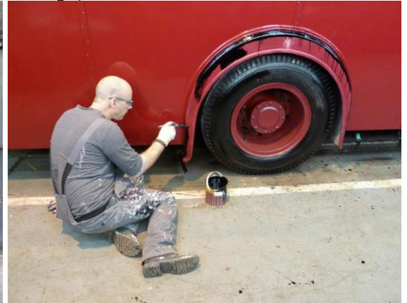
Above: Steve the painter applying black paint to 375's mudguards (29 April)
