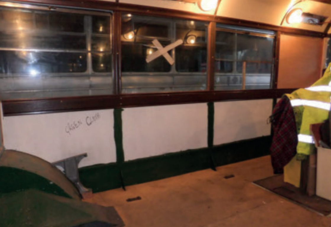
A close-up of the newly-varnished window frames in the lower saloon, showing the refitted glazing and panelling above and below the windows
