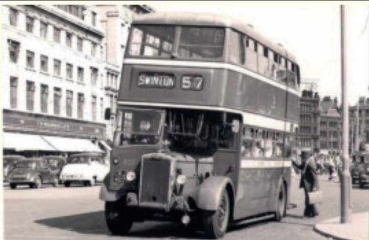
Salford 407 was one of 195 similar Daimler CVG6 with MCCW H54R bodies delivered in 1950-1. Salford started operation on the 57/ 77 with these buses and they were only displaced in 1962 by Salford's next delivery of new buses. No.407 is in Piccadilly heading towards Swinton before the introduction of the one-way system, but has lost its original silver roof, which dates the photo to the mid-fifties
