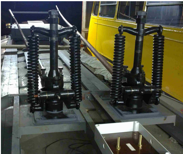
Left: a close-up view of the newly-manufactured trolley gear on the roof of 73
