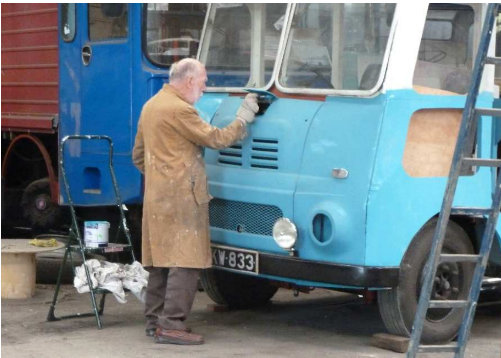
Stanley applying blue undercoat to the bonnet of Andy Feather's Bradford tower wagon 033 at the Keighley Bus Museum
