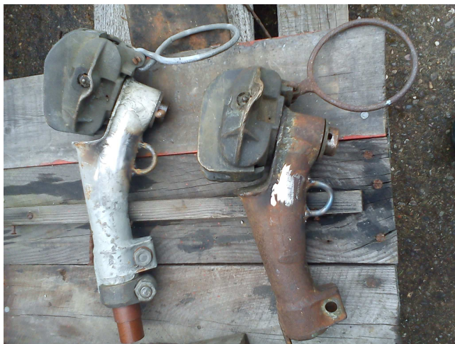
Re-engineered trolley heads angled at 30 degrees Photo: Mike Johnson
