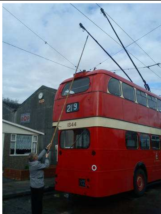
Dave Croft assists in earth-leakage testing, of 1344, before service begins: here he is lowering the negative boom Photo: Mike Johnson
