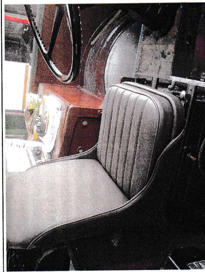
1348's newly upholstered driver's seat in place in a substantially-finished cab Photo: John Crossley
